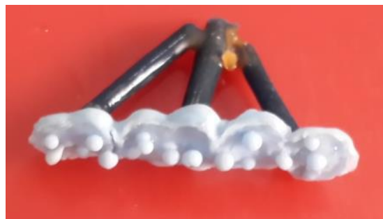
Figure - 8 :- Sprue attached to wax pattern.
